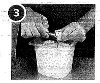
Adjust the thermometer so it reads 32°F (0°C).
