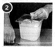
Put the thermometer stem or probe into the ice water.
